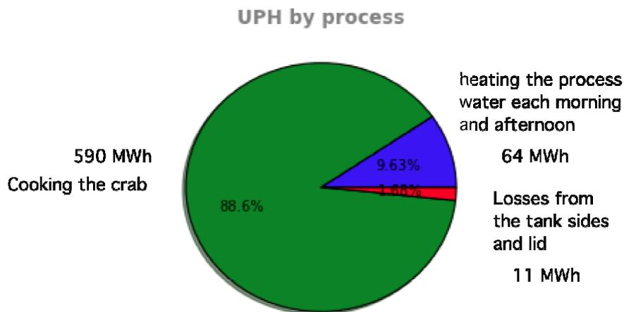
Following on from the site audit, the company has since insulated the walls of one of the two crab cooking vessels, and plans to do the same for the second vessel at the end of 2011 during Christmas shut-down. Thus, the above losses will be reduced by up to 90% based on the thickness of the insulation installed.
